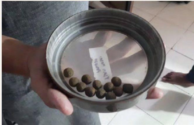
Specimens made using the tablet machine
