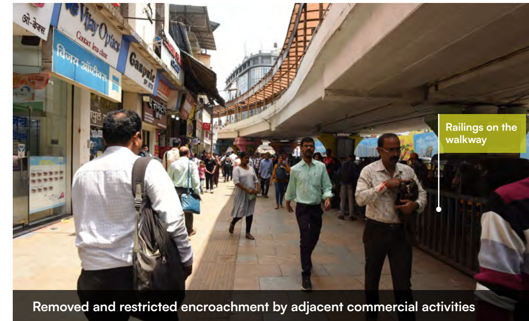
Unlike the other projects in the ABD project, Shahabad stone was used for the footpath in this stretch keeping in mind the high pedestrian volumes
